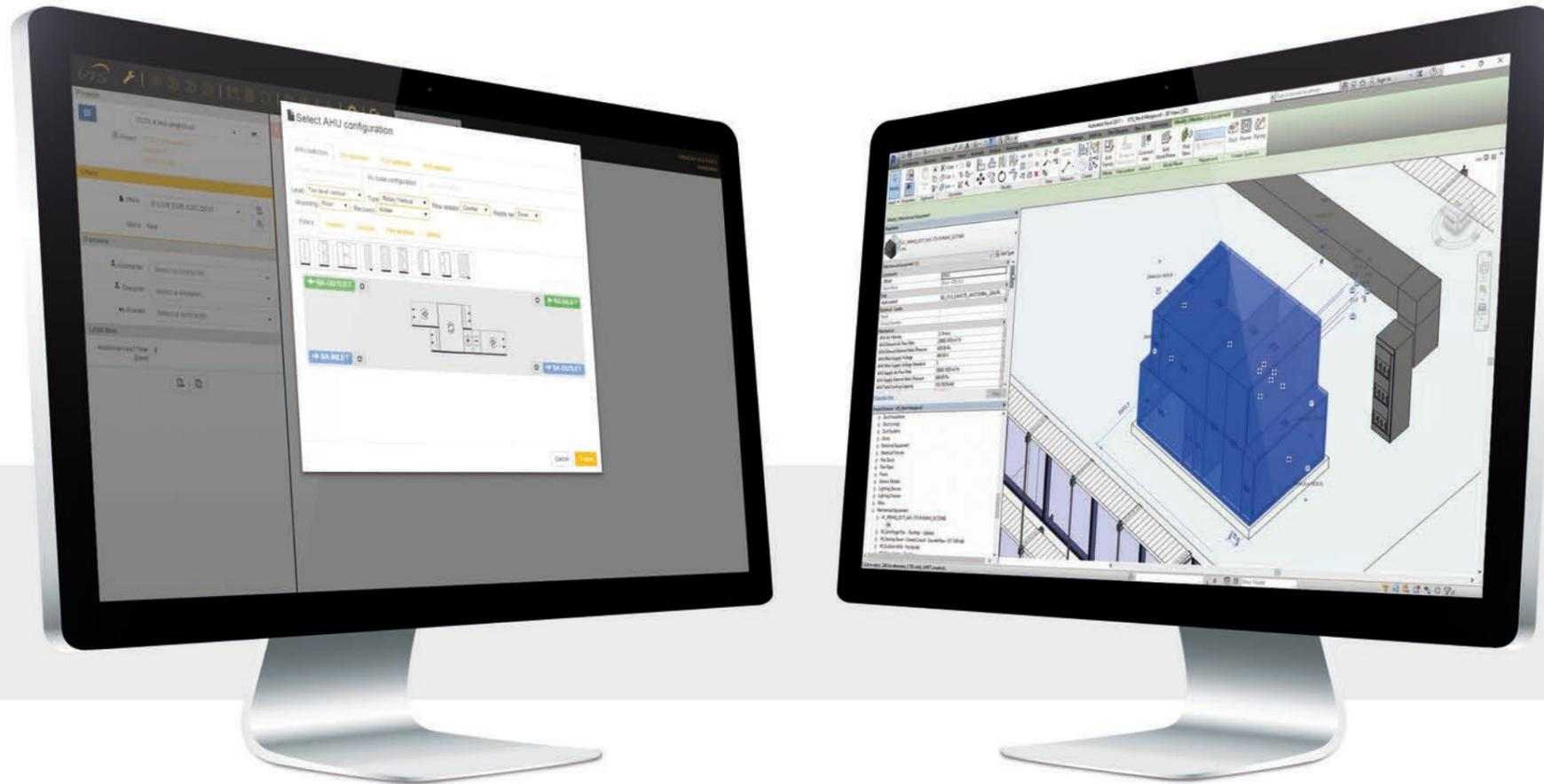
The release of so called families for the Autodesk Revit® environment by VTS makes it easier to design agencies to model the building installations on the basis of using the same platform. At present the on-line generator is a unique solution in BIM environment. It enables the generation of a VENTUS air-handling unit model practically in no time in any configuration and with any parameters.
